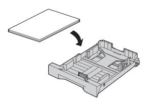
Insert the paper input tray to the unit, lifting the front part of the tray. Then push it completely into the unit.
